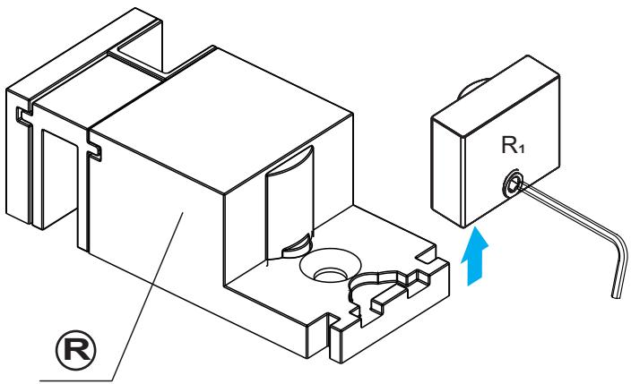
Remove Part R<sub>1</sub> to Secure the Sliding Glass Panel (G) in Step 10.2
