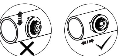
Ensure the curved surface of the Fixed Panel Bracket (I) fits snugly against the Top Track (F)
