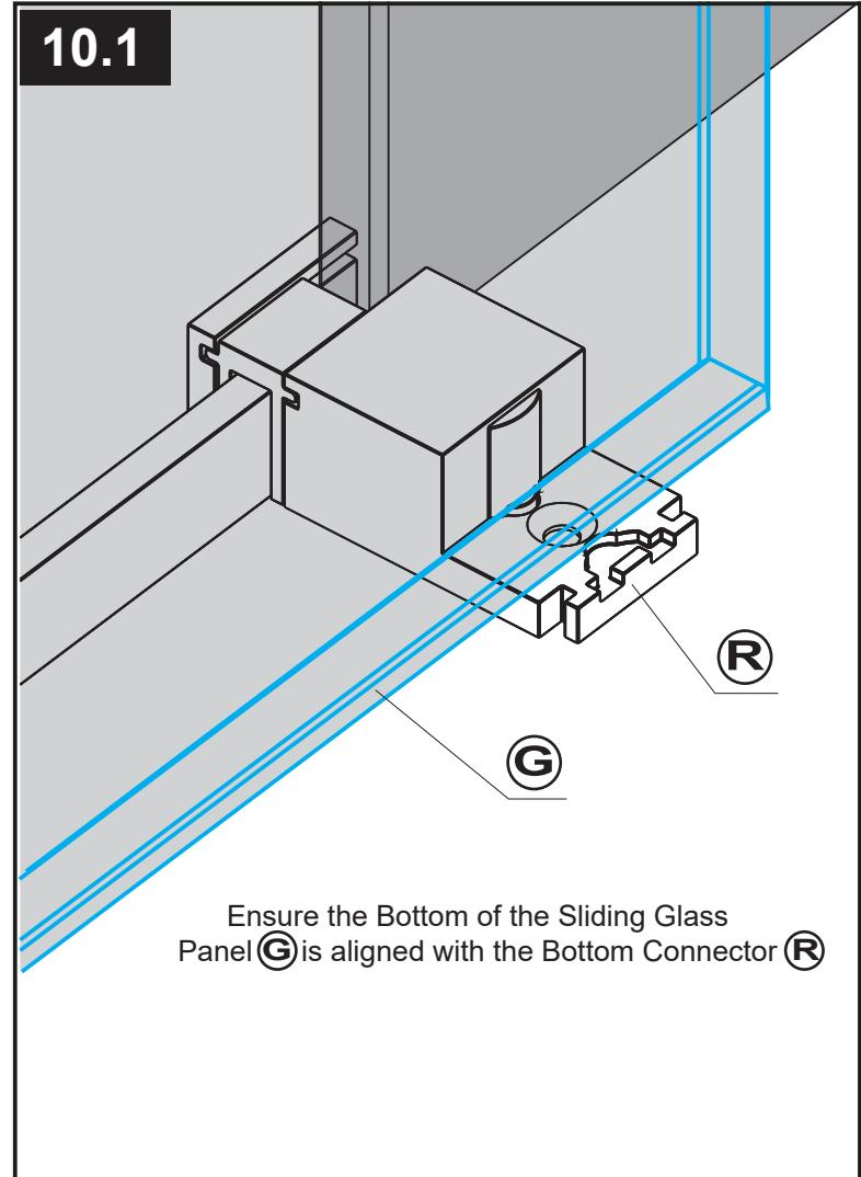
Ensure the Bottom of the Sliding Glass Panel **G** is aligned with the Bottom Connector **R**
