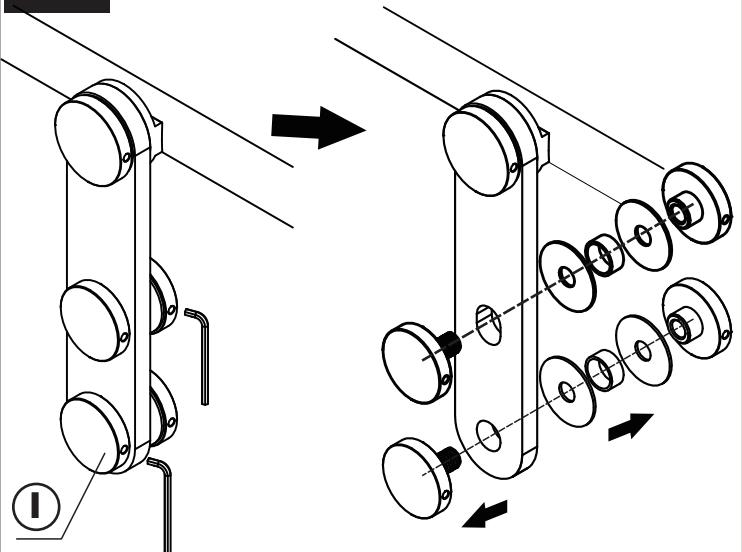
Disassemble Fixed Panel Bracket (I)
