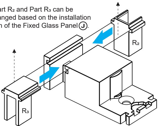
Part R<sub>2</sub>: Used to Secure the Fixed Glass Panel (J) in Place
