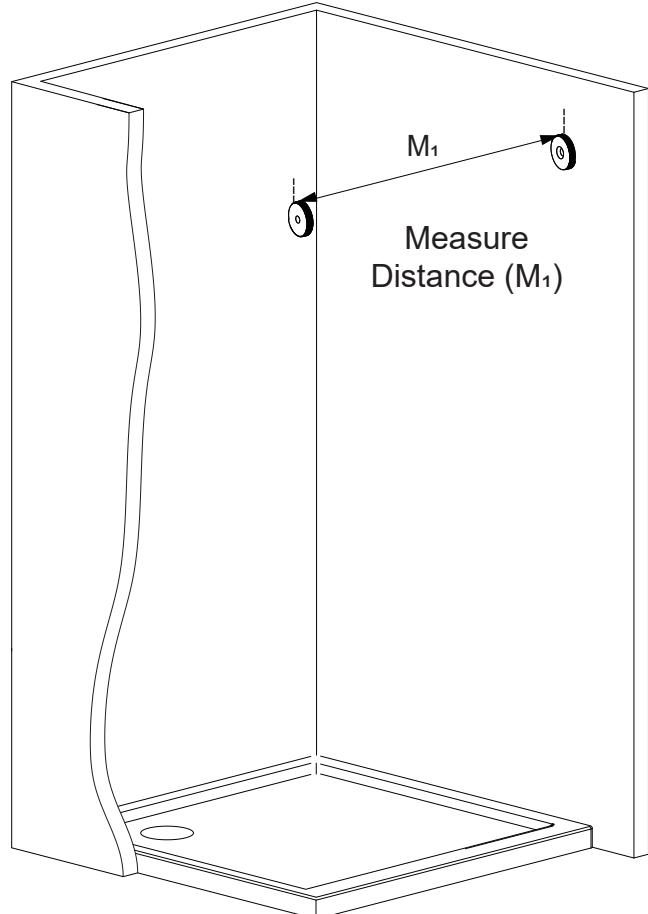
THE INSTALLATION SHOWN IS BASED ON PLUMB FINISHED WALLS AND A LEVELLED BASE. IF THESE CONDITIONS ARE NOT MET, PLEASE ADJUST ACCORDINGLY.
