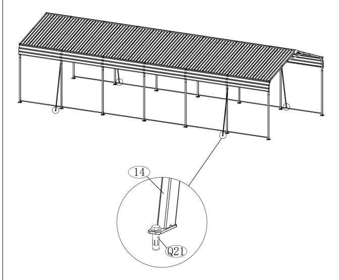
1. It is necessary to use ground nails and expansion screws, whether installed on stable ground, to avoid the collapse of the car shed to the inside or nearby personnel causing devastating injuries and property losses.
