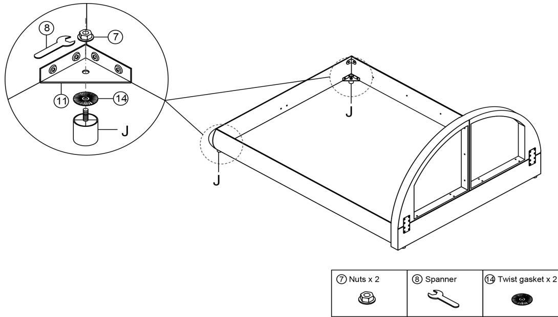
Attach the Bed legs J to the Metal Corner ⑪ with Nuts ⑦ and Twist gasket ⑭ by using Spanner ⑧.
