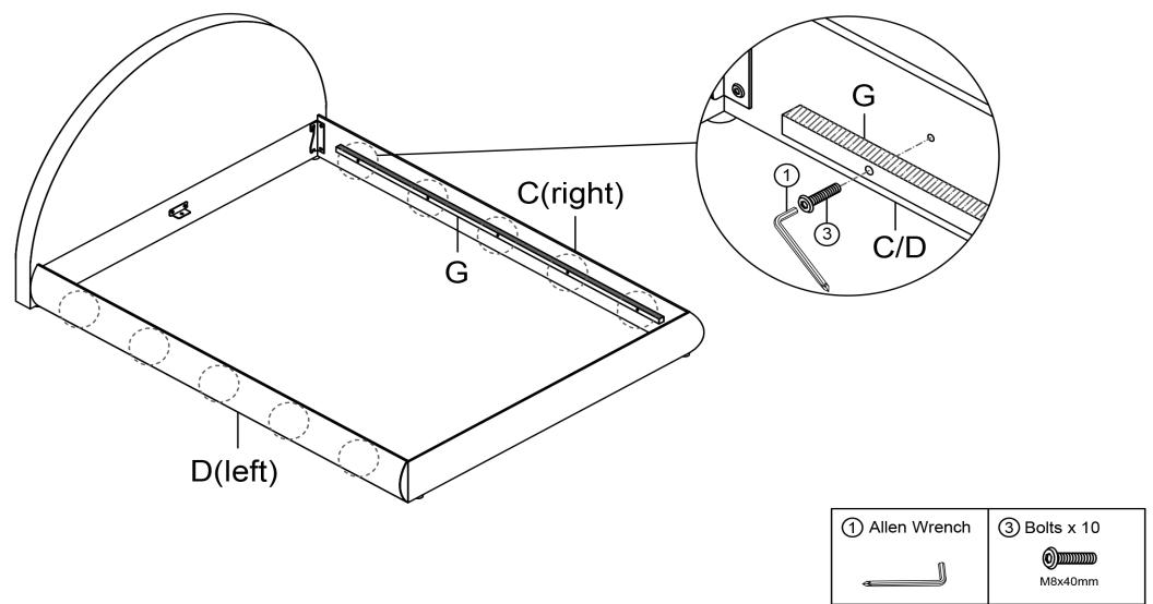
Attach the Side rails support bar G to the Side rail C(right) and Side rail D(left) with Bolts ③ by using Allen Wrench ①.
