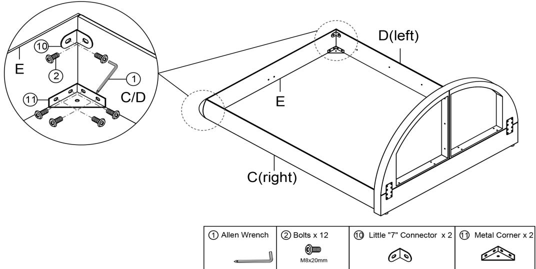
Attach the Foot board E to the Side rail C(right) and Side rail D(left) with Bolts ②, Little "7" Connector ⑩ and Metal Corner ⑪ by using Allen Wrench ①.
