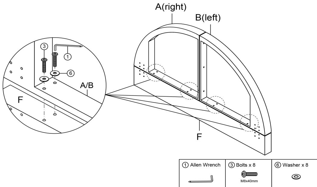
Attach the Base head board F to the Top head board A(right) and Top head board B(left) with Bolts ③ and Washer ⑥ by using Allen Wrench ①.
