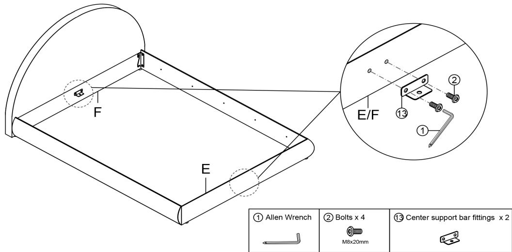
Attach the Center support bar fittings ⑬ to the Foot board E and Base head board F with Bolts ② by using Allen Wrench ①.
