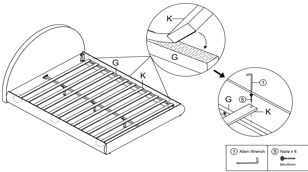
Attach the Slats K to the Side rails support bar G with Nails ⑤ by using Allen Wrench ① or electrical drill .
