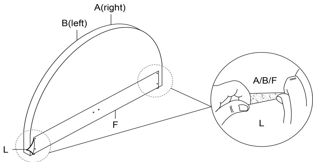
Stick the Bedhead cover L onto the Top head board A(right) ,Top head board B(left) and Base head board F.
