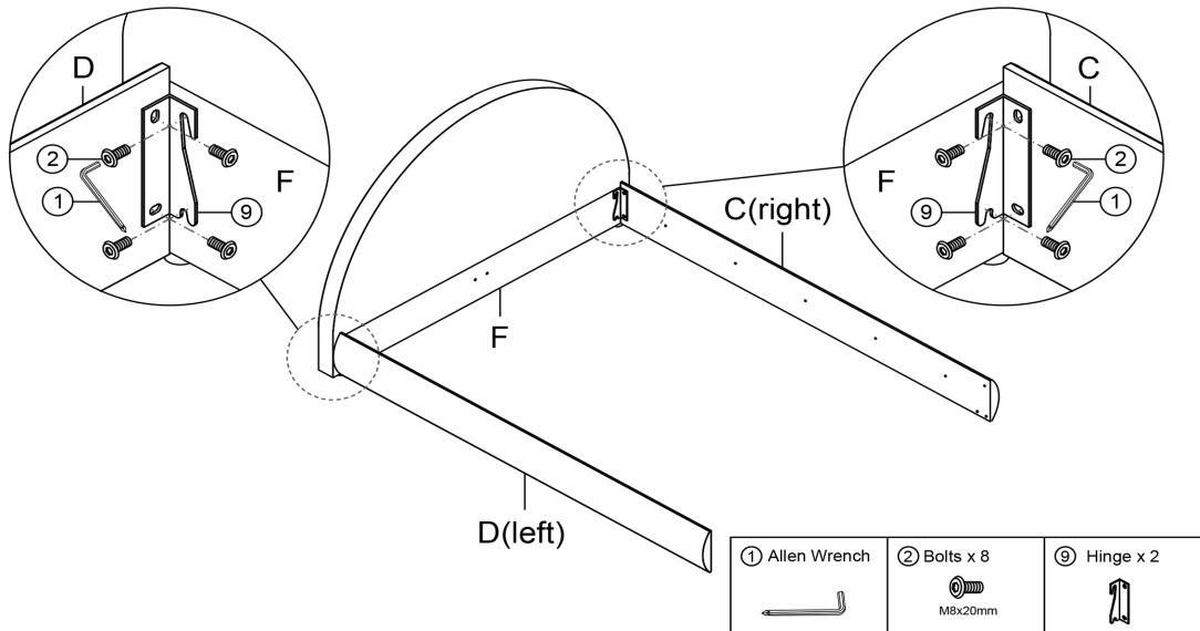
Attach the Side rail C(right) and Side rail D(left) to the Base head board F with Bolts ② and Hinge ⑨ by using Allen Wrench ①.
