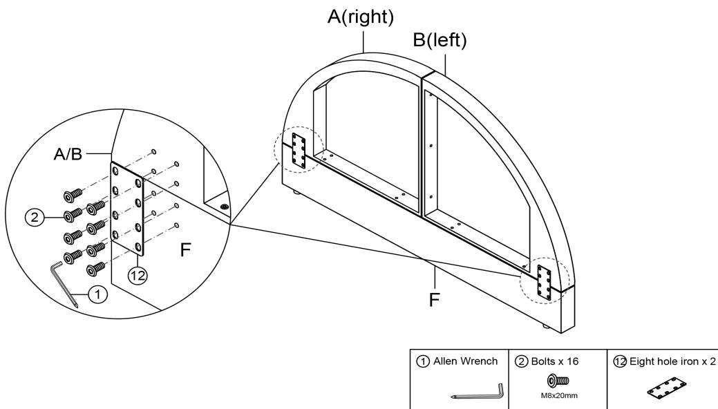
Attach the Base head board F to the Top head board A(right) and Top head board B(left) with Bolts ② and Eight hole iron ⑫ by using Wrench ①.
