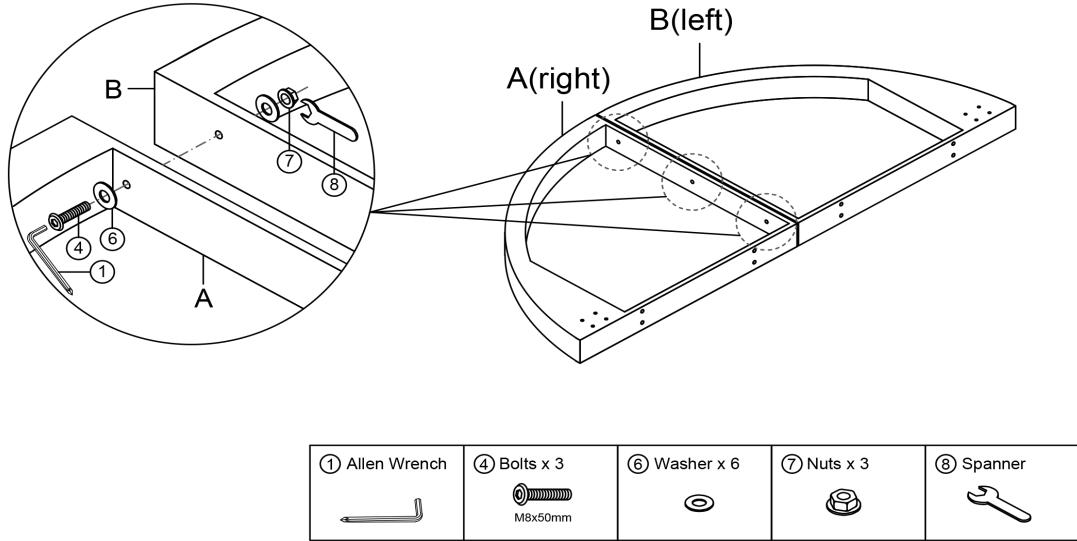
Attach the Top head board A(right) to the Top head board B(left) with Bolts ④, Washer ⑥ and Nuts ⑦ by using Allen Wrench ① and Spanner ⑧.
