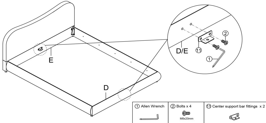
Attach the Center support bar fittings ⑪ to the Foot board D and Base head board E with Bolts ② by using Allen Wrench ①.
