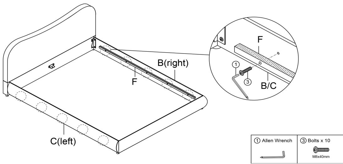
Attach the Side rails support bar F to the Side rail B(right) and Side rail C(left) with Bolts ③ by using Allen Wrench ①.
