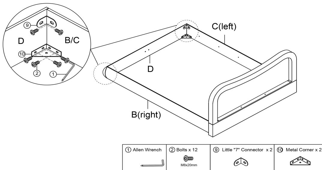
Attach the Foot board D to the Side rail B(right) and Side rail C(left) with Bolts ②, Little "7" Connector ⑨ and Metal Corner ⑩ by using Allen Wrench ①.
