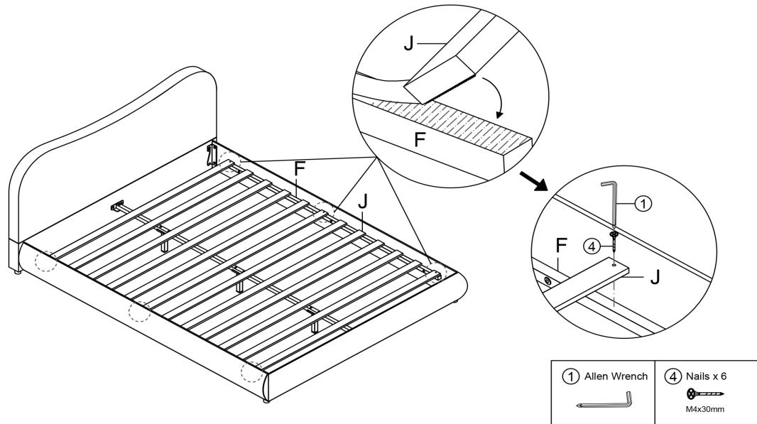
Attach the Slats J to the Side rails support bar F with Nails ④ by using Allen Wrench ① or electrical drill .
