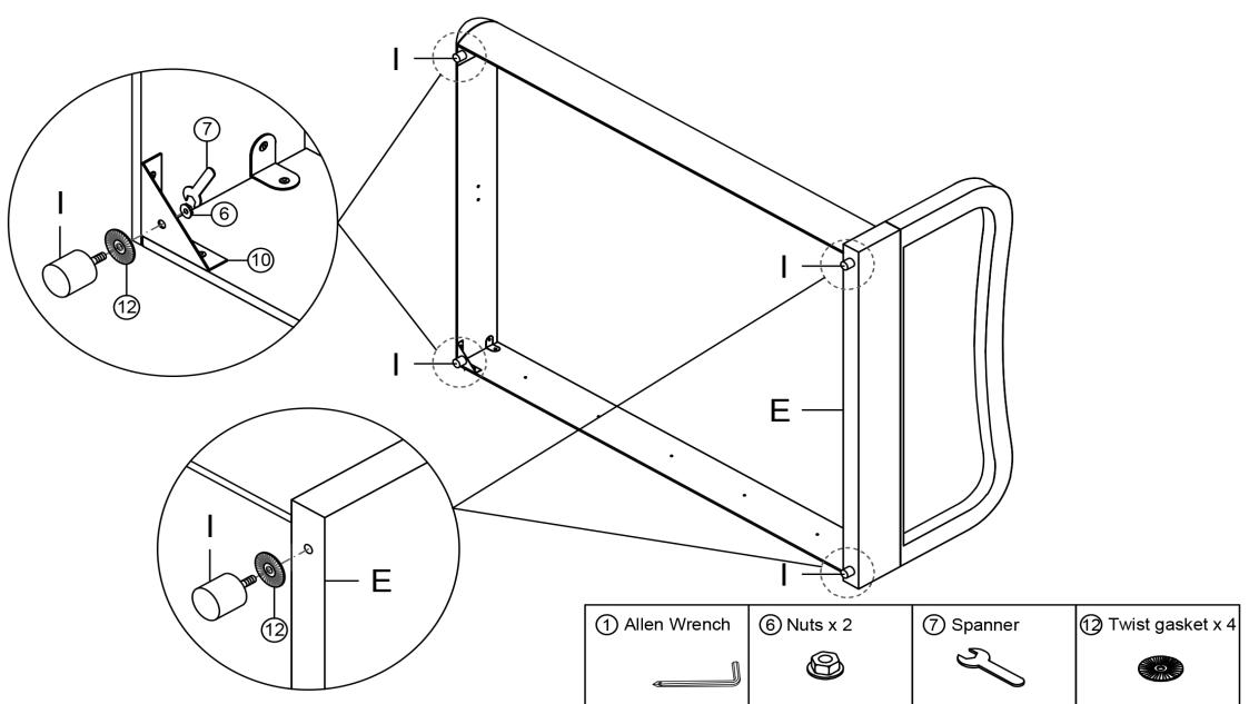
Attach the Bed legs I to the Base head board E and Metal Corner ⑩ with Nuts ⑥ and Twist gasket ⑫ by using Spanner ⑦.
