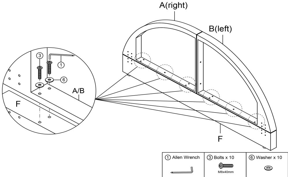
Attach the Base head board F to the Top head board A(right) and Top head board B(left) with Bolts ③ and Washer ⑥ by using Allen Wrench ①.
