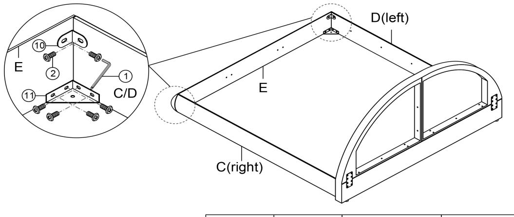
Attach the Foot board E to the Side rail C(right) and Side rail D(left) with Bolts ②, Little "7" Connector ⑩ and Metal Corner ⑪ by using Allen Wrench ①.
