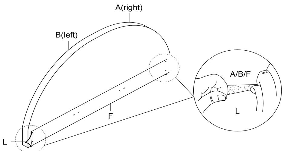
Stick the Bedhead cover L onto the Top head board A(right) ,Top head board B(left) and Base head board F.
