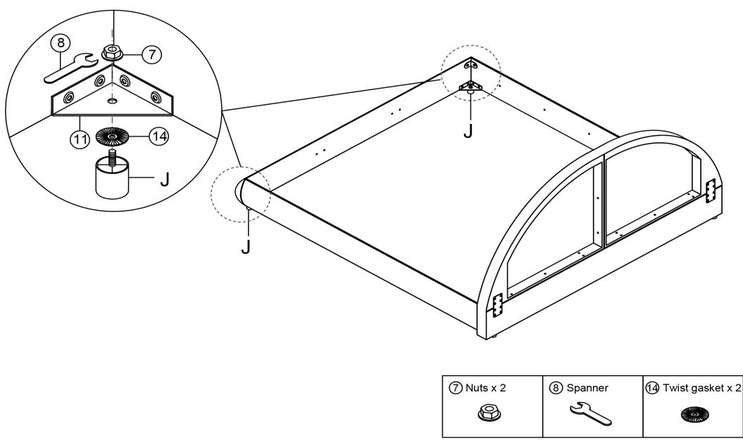
Attach the Bed legs J to the Metal Corner ⑪ with Nuts ⑦ and Twist gasket ⑭ by using Spanner ⑧.
