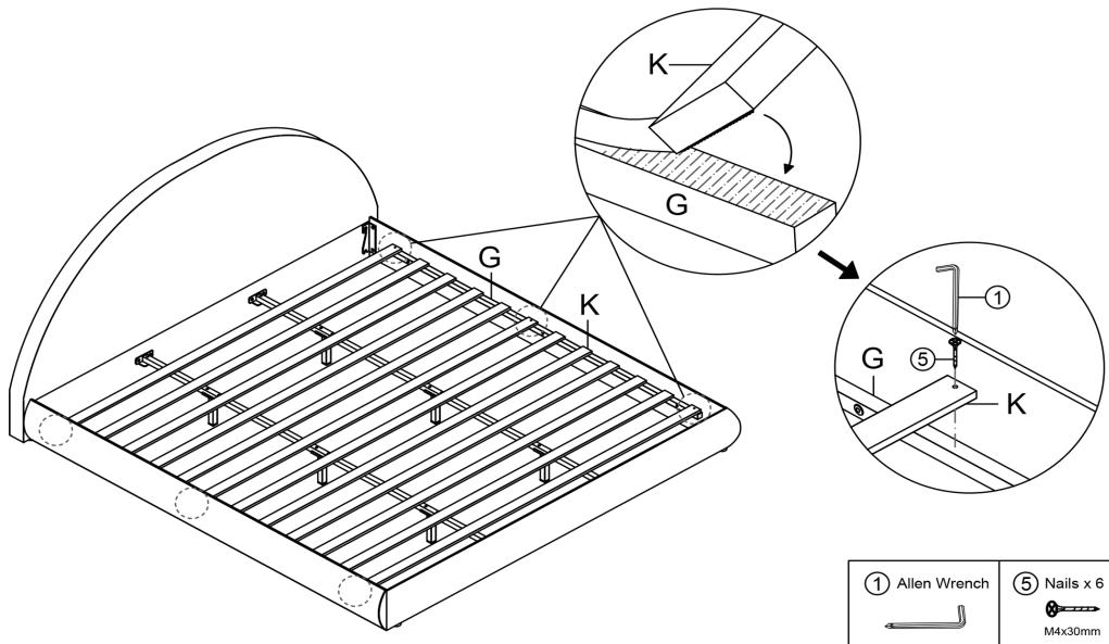
Attach the Slats K to the Side rails support bar G with Nails ⑤ by using Allen Wrench ① or electrical drill .
