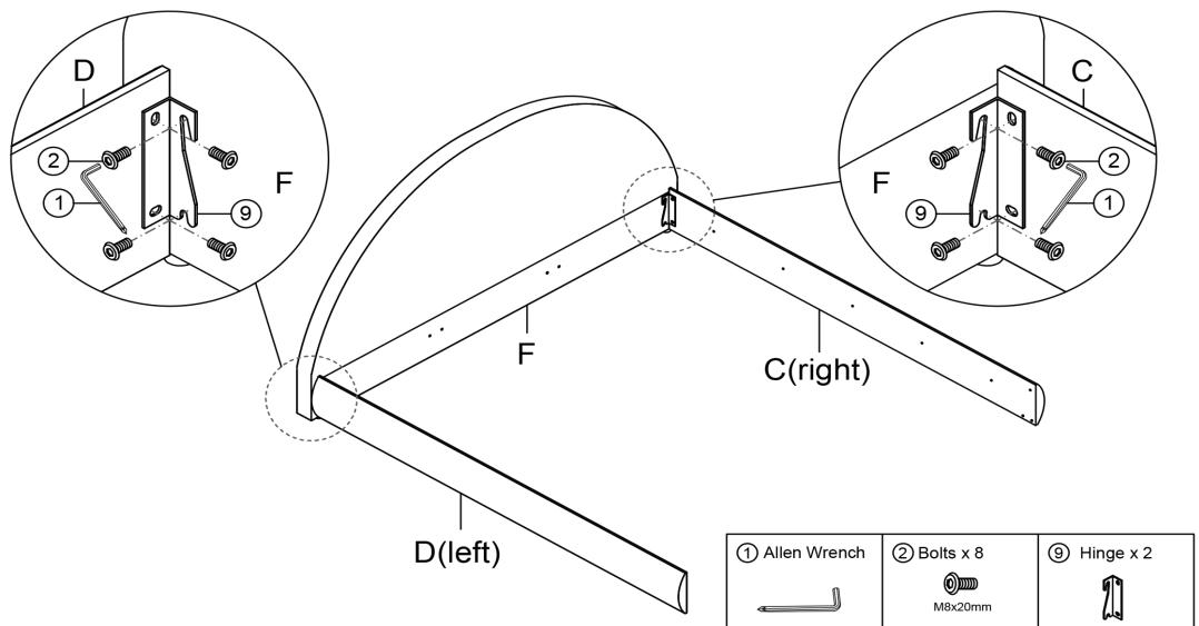
Attach the Side rail C(right) and Side rail D(left) to the Base head board F with Bolts ② and and Hinge ⑨ by using Allen Wrench ①.
