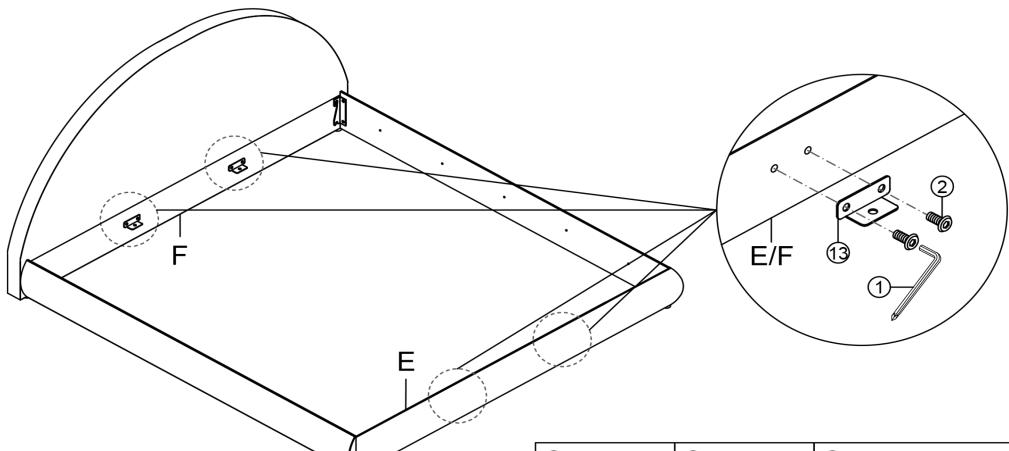
Attach the Center support bar fittings ⑬ to the Foot board E and Base head board F with Bolts ② by using Allen Wrench ①.
