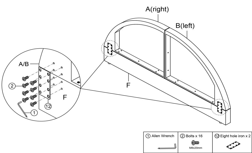
Attach the Base head board F to the Top head board A(right) and Top head board B(left) with Bolts ② and Eight hole iron ⑫ by using Wrench ①.
