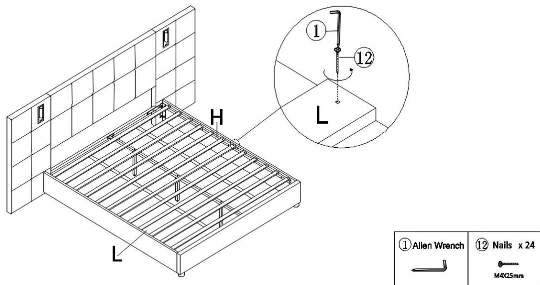
Fix the Slats (L) to the side support bar (H) with Nails(⑫) by using Allen Wrench(①) or Electric drill.
