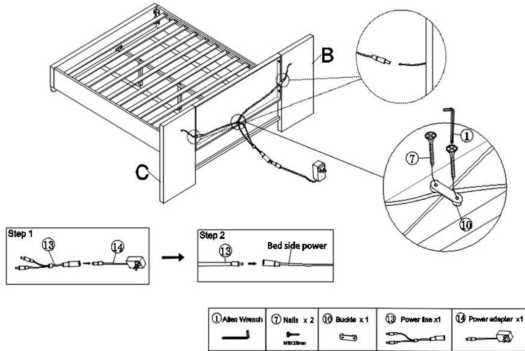
At first, connect the Power adapter (⑭) to the Power line(⑬) .
