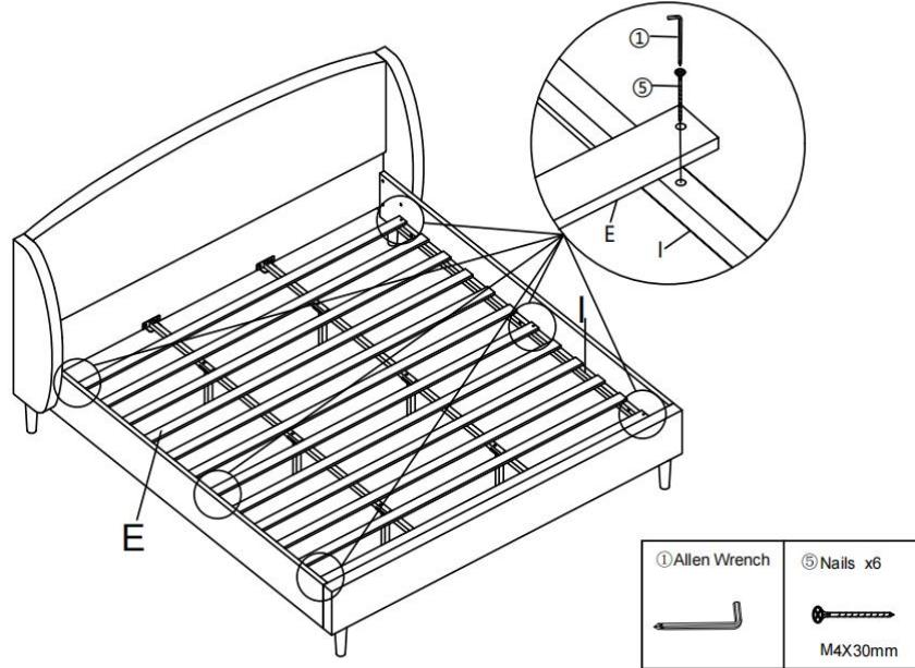
Attach the Slats E to the Side rails support bar I with Nails ⑤ by using Allen Wrench ①.
