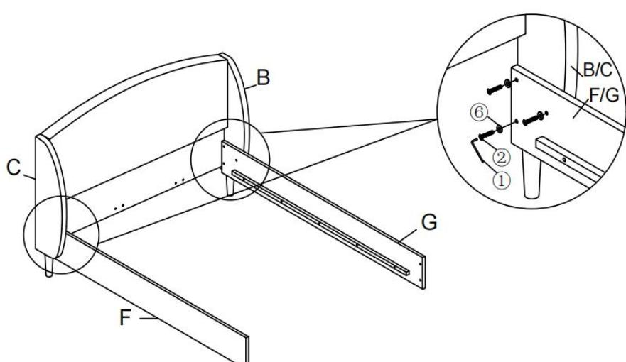
Attach the Side rail F and G to the Side head board B and C with Bolts ② and Washer ⑥ by using Allen Wrench ①.
