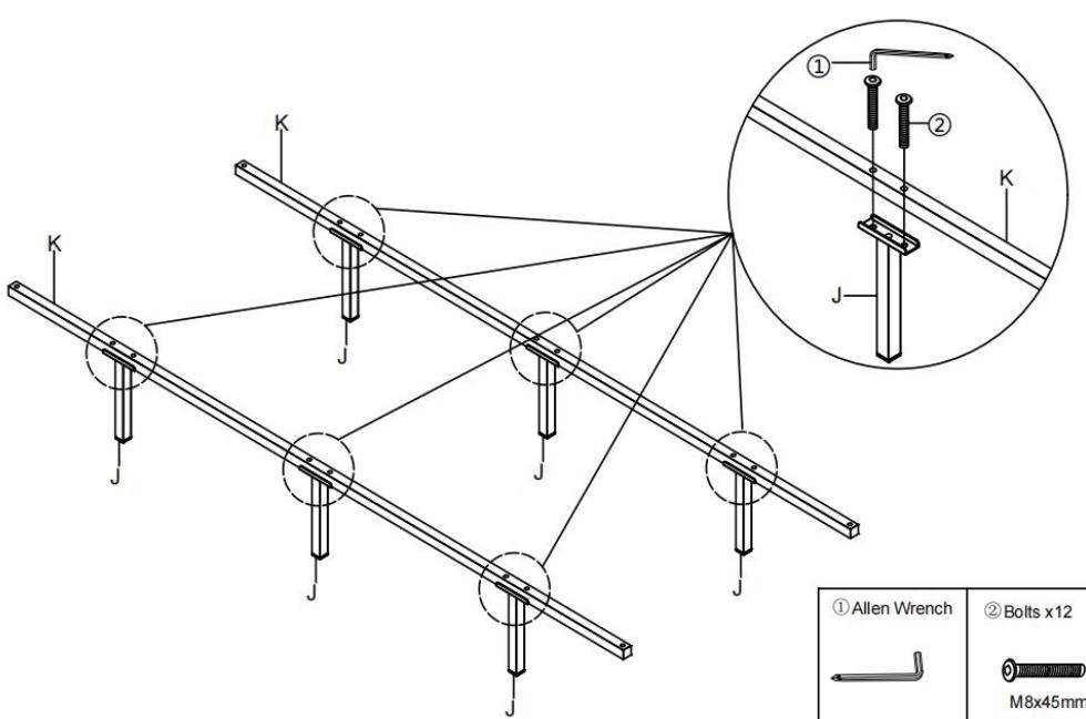
Attach the Middle support leg J to the Center support bar K with Bolts ② by using Allen Wrench ①.
