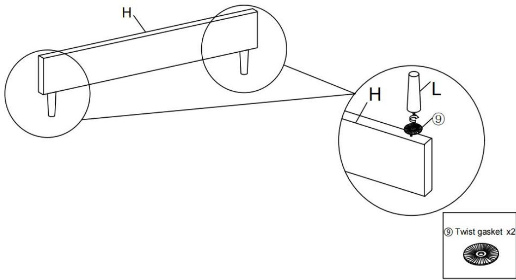
Attach the Support leg L to the Foot board H with Twist gasket ⑨.
