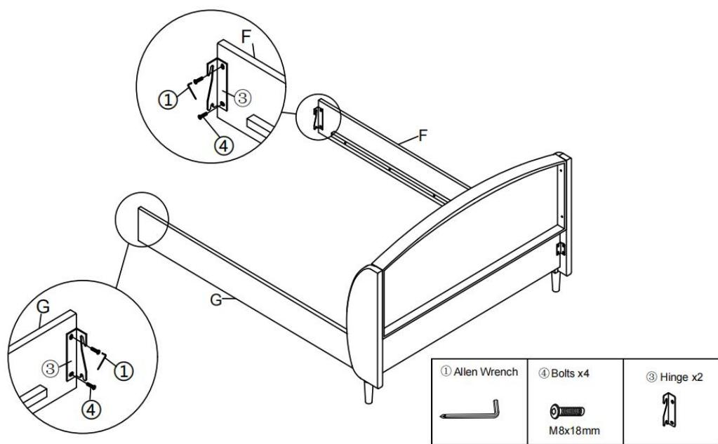
Attach the Hinge ③ to the Side rail G and F with Bolts ④ by using Allen Wrench ①.
