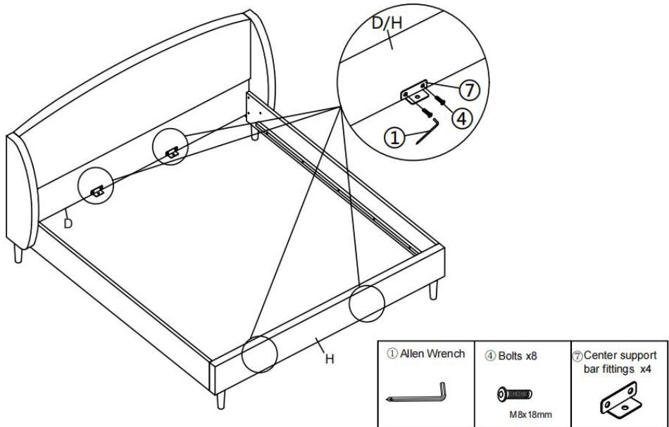
Attach the Center support bar fittings ⑦ to the Bottom board D and Foot board H with Bolts ④ by using Allen Wrench ①.
