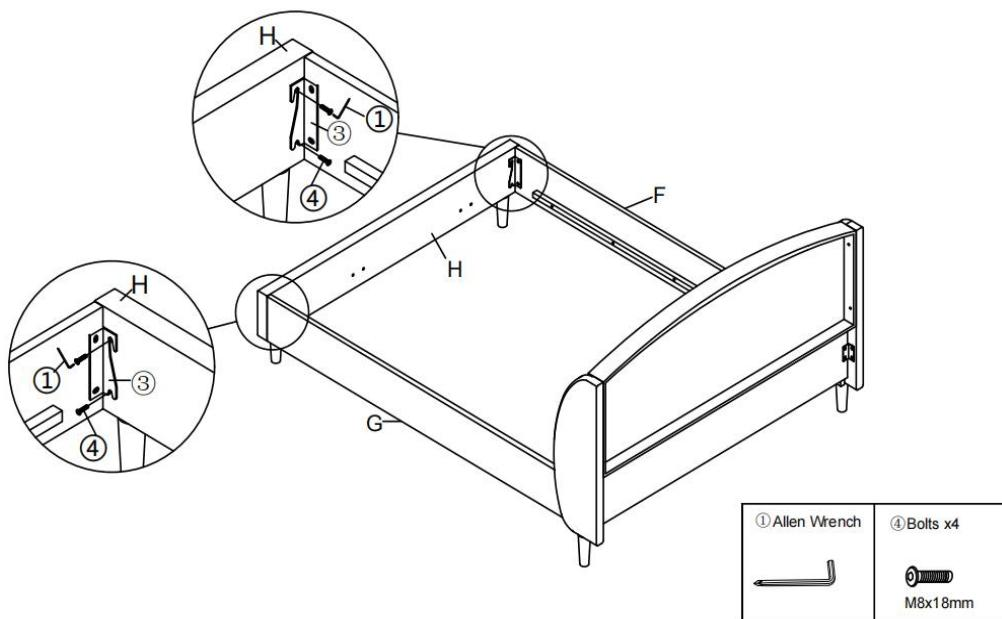
Attach the Foot board H to the Hinge ③ with Bolts ④ by using Allen Wrench ①.
