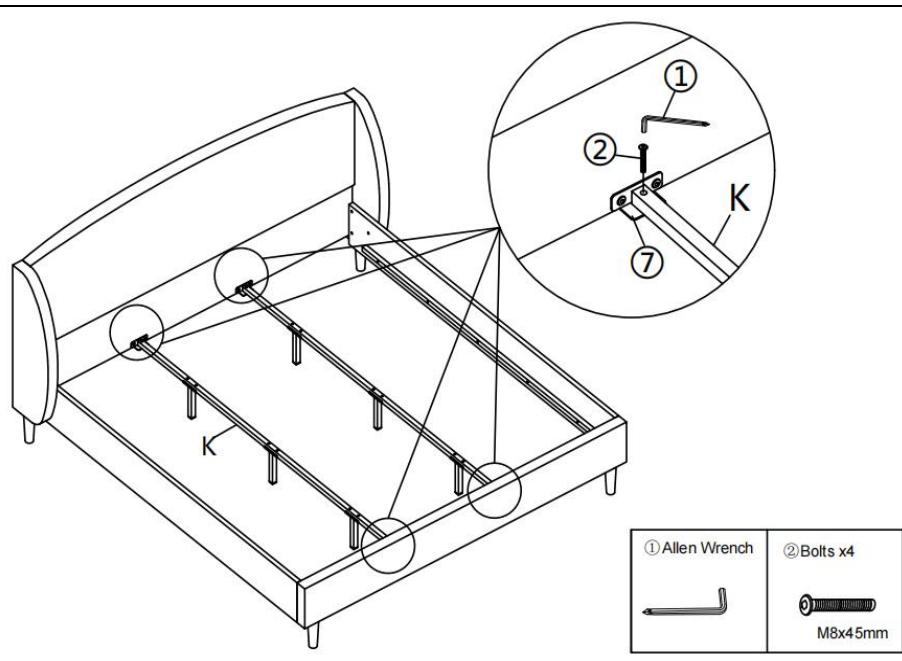
Attach the Center support bar K to the Center support bar fittings ⑦ with Bolts ② by using Allen Wrench ①.
