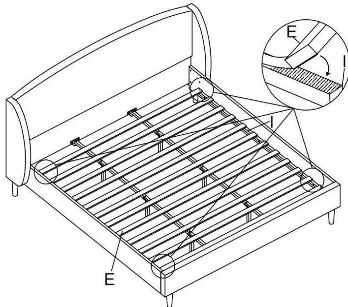
Put the Slats E on the Side rails support bar I.
