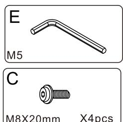
Attach the Hinge (⑬ /⑭) to side rail (⑥ /⑦) with Bolts (⑩) by using Allen Wrench (E).
