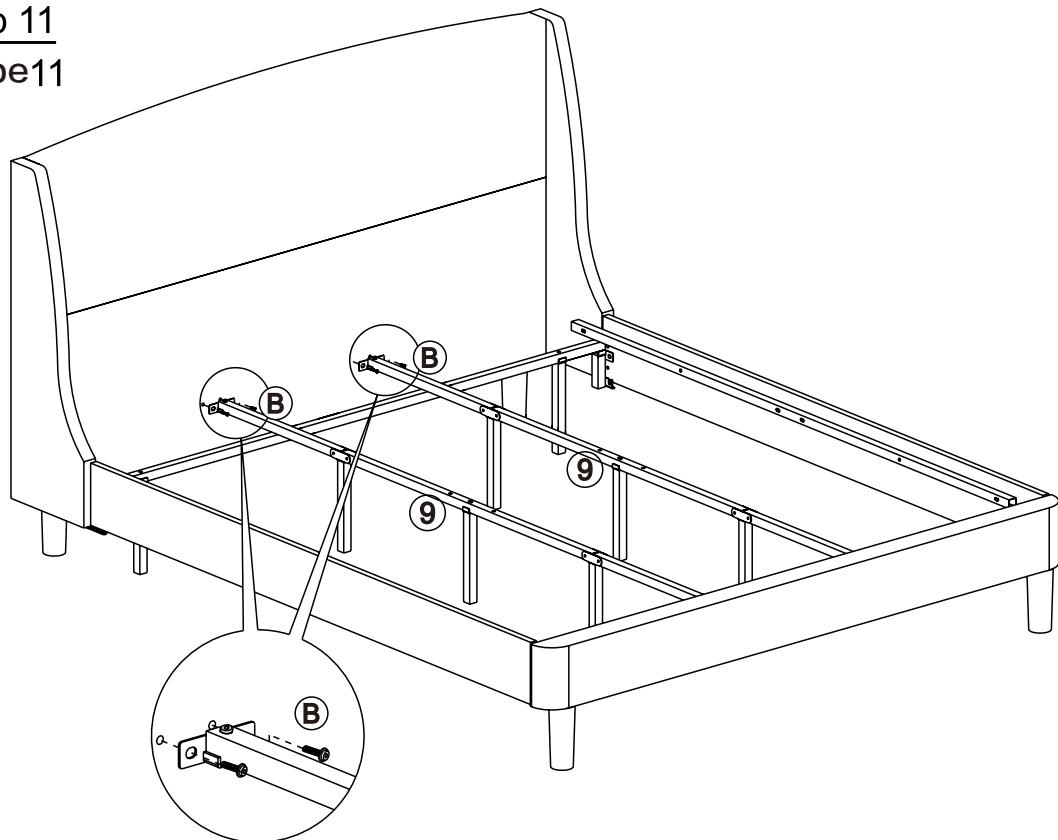
Attach the Center support bar fitting (12) to Headboard (2) with Bolts(B) by using Allen Wrench(E).
