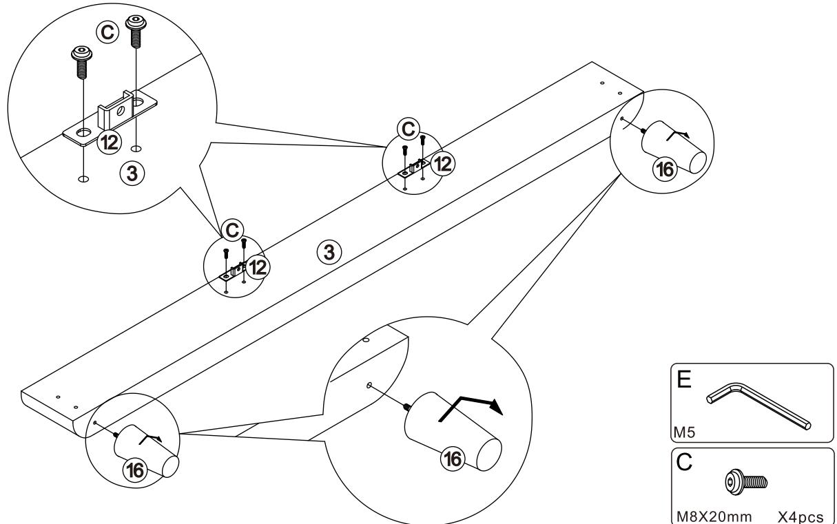
Attach the Center support bar fitting (12) and Bed leg (16) to Foot board (3) with Bolts(C) by using Allen Wrench(E).
