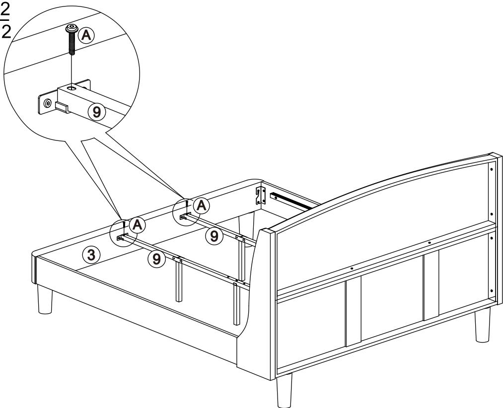
Attach the Center support bar(9) to Center support bar fitting(12) with Bolts (A) by using Allen Wrench(E).
