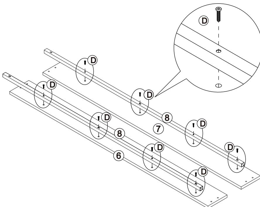
Attach the Side rails support bar (⑧) to side rail (⑥/⑦) with Bolts (⑩) by using Allen Wrench (F).
