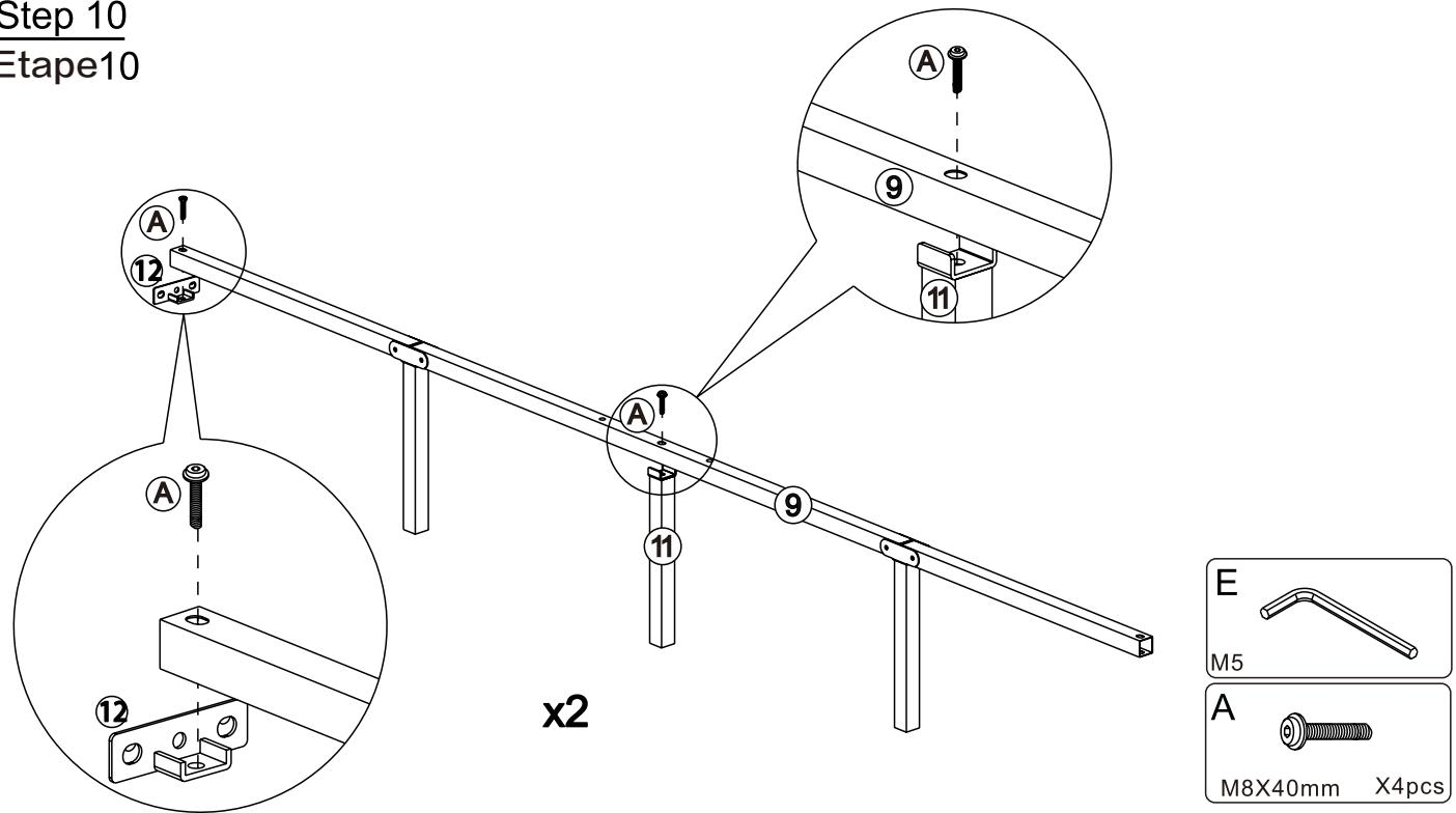
Attach the Center support bar(9) to Middle support leg(11) and Center support bar fitting (12) with Bolts(A) by using Allen Wrench(E).
