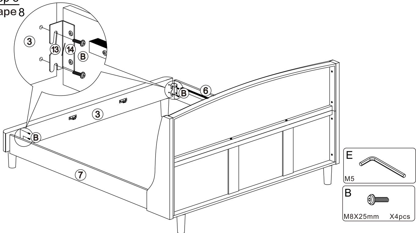
Attach the Foot board (3) to Side rail (6)/(7) with Hinge (13)/(14) and Bolts (B) by using Allen Wrench (E).
