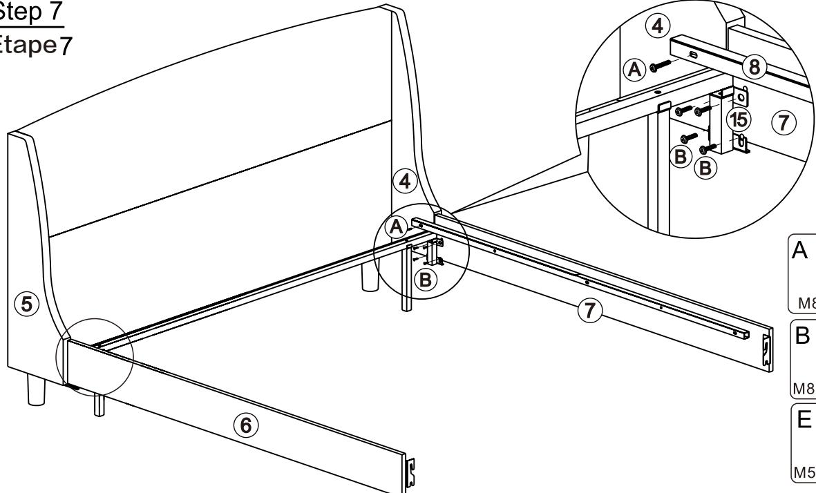
Attach Side flank connection (15) to Side rail (6)/(7) with Bolts (A)/(B) by using Allen Wrench (E).
