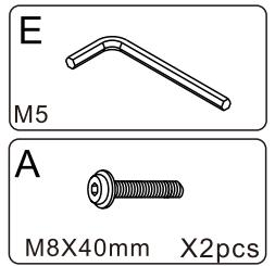
Attach the Headboard (①) to Headboard (②) with Bolts (Ⓐ) by using Allen Wrench (Ⓔ).
