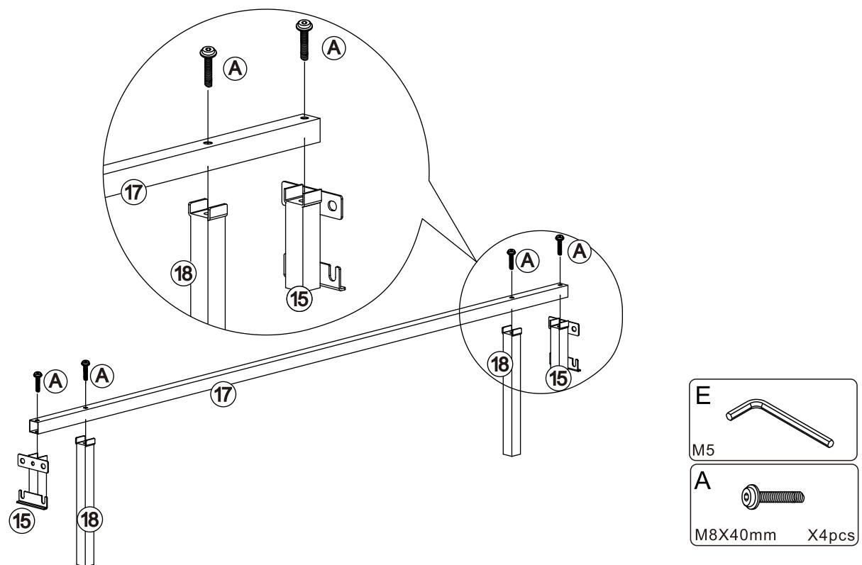
Attach the Side flank horizontal pipe (17) to Horizontal pipe support leg(18) and Side flank connection(15) with Bolts(A) by using Allen Wrench(E).
