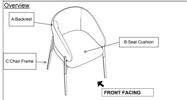
This dining chair has multiple parts and may require up to 30 minutes to assemble. To give you an overview of the dining chair, the above picture is to help you put the various parts into perspective. Please read through the instructions herebelow to familiarise the parts and steps before assembly.
