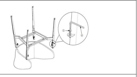
Connect the chair frame (C) and the backrest (A) together. Use the Allen key (4) to tighten the Allen screw (1).
