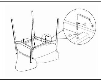
Connect the chair frame (C) and the seat (B) together. Use the Allen key (4) to tighten the Allen screw (2) with the washer (3) in place.
