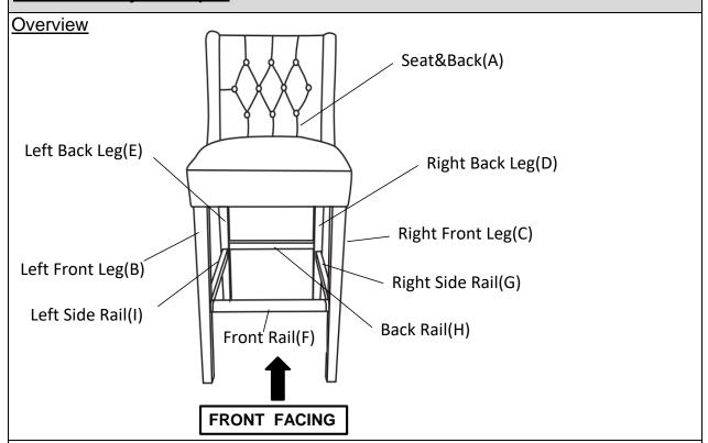
This Bar Chair has multiple parts and may require up to some 30 minutes to assemble. To give you an overview of the Bar Stool parts, the above picture is to help you put the various parts into perspective. Please read through the instructions herebelow to familiarise the parts and steps before assembly.
