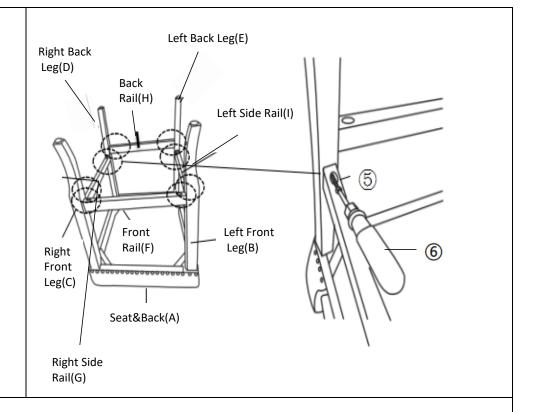
Insert the Side Rail (G) into round housing of the Right Back Leg (D) as shown above.
